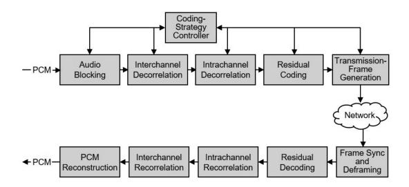
Figure 2. Qualcomm aptX Lossless codec. The technology uses both audio and environmental information. The coding-strategy controller collects real-time statistics, optimizing the encoding process on the basis of time-domain audio analysis, including sample amplitudes and sample correlation between and within channels, as well as environmental parameters such as Bluetooth link quality.
