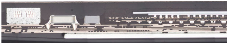
Cross-section view of the Apple S1 chip from an Apple Watch Series 1. PHOTO: CHIPWORKS
